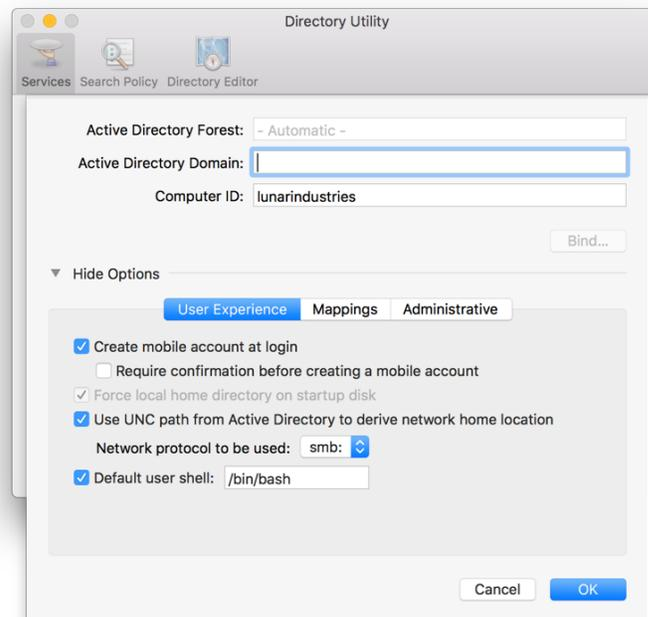
2. Deploy the Mobile-SmartcardLogin.plist to the Mac, allowing any user with a valid Smart card to build a Mobile User Account.
